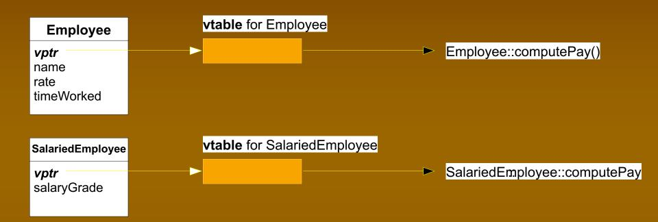
Each class has a *vtable* (pointers to its virtual functions)
